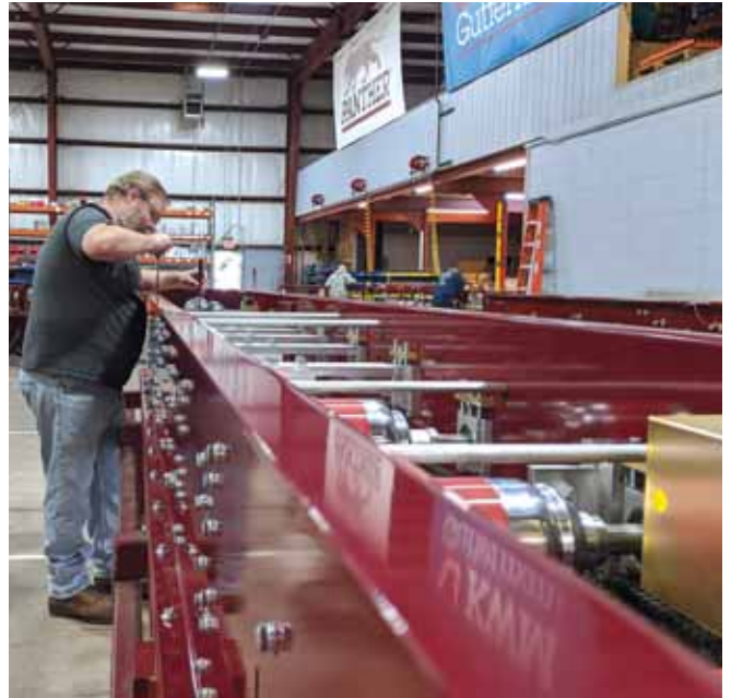
A worker at KWM Gutterman prepares another roll former for market. Photo provided by KWM Gutterman
