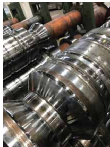
When rolls are worn out, a catastrophic event is soon to follow, causing tools to run together and double sheeting of material to occur.
