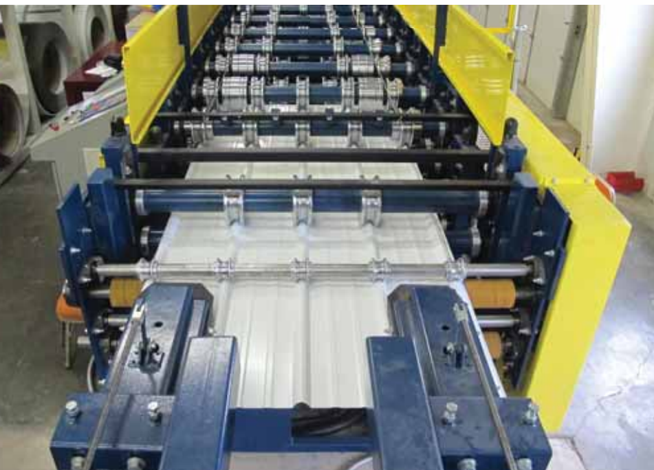
(BELOW) Rush River installed its second MRS Titan II roll former last year, used for making the ApexX4 and Summit panels. RUSH RIVER STEEL PHOTOS
