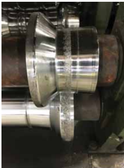
When rolls are worn out, a catastrophic event is soon to follow, causing tools to run together and double sheeting of material to occur.
