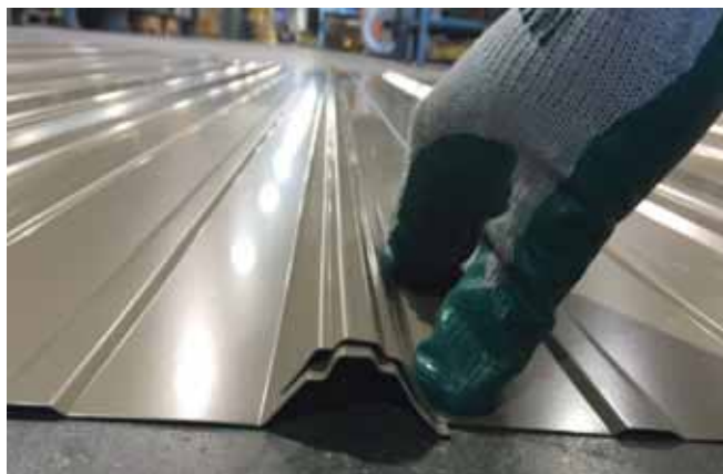
Overlap control determines how weathertight a panel will be. Loss of crisp bends is a sign of tooling wear.
