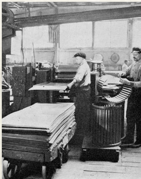
This 1931 photo inside the Wheeling Corrugating factory in Wheeling, West Virginia, shows an early shop-based machine that was used to corrugate metal panels for the use in making trash cans. PHOTO COURTESY OF THE OHIO COUNTY PUBLIC LIBRARY ARCHIVES, WHEELING, WEST VIRGINIA.
