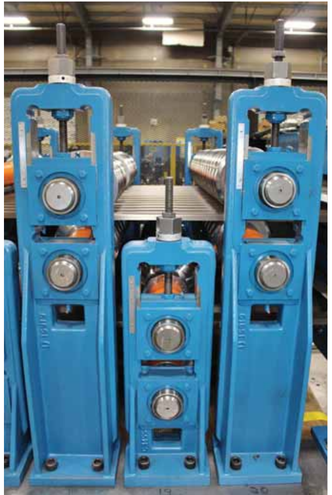
This photo shows the standard configuration of a dual profile machine, with upper and lower stands. A single profile needs only one level of stands. ASC MACHINE TOOLS PHOTO
