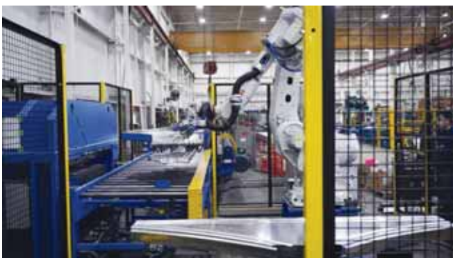
Robotic technology is making its way into roll forming to help provide quicker orientation between operations.
