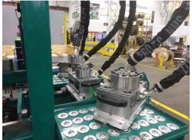
Some manufacturers attach conveyor tables to the press where dies can be stored.
