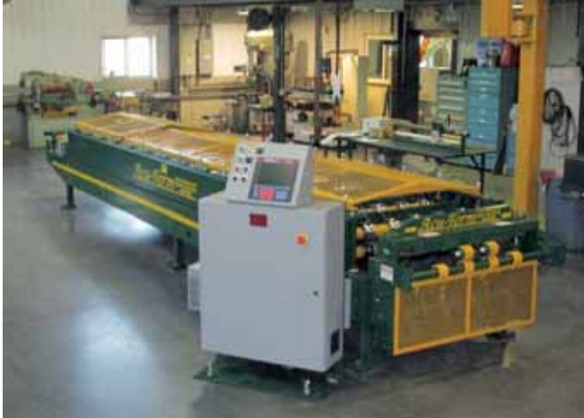
Acu-Form Equipment has found a favorable market for its single profile roll former that forms a combo panel, satisfying dual needs.
