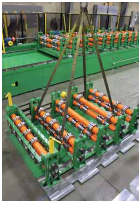
This subplated machine shows the typical configuration of a multiple profile machine. ASC MACHINE TOOLS PHOTO
