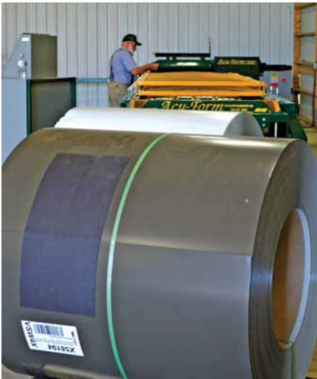
Your Quality Metal sources its steel from both Progressive Metals and United Steel Supply. Here, a roll of Zincoalume waits to be among the first off the new line.
