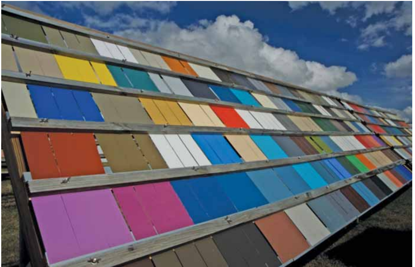
This paint fence at the Sherwin-Williams Coil Coatings A2LA testing facility in Ft. Myers, Florida, has provided natural exposure testing for 52 years.
