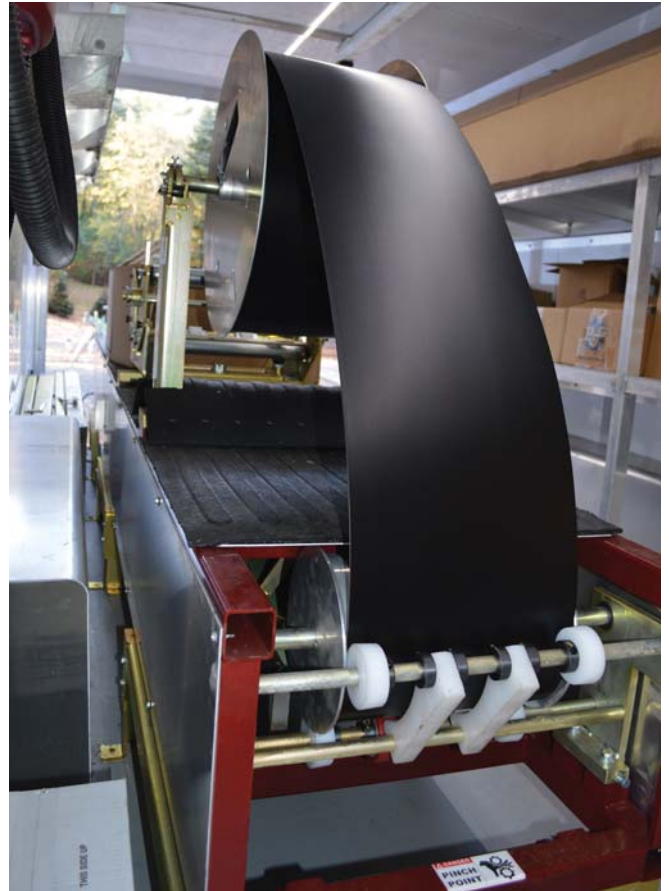
This KWM Gutterman half round roll former was on a jobsite cranking out 184' of black aluminum gutter for a vacation home.
