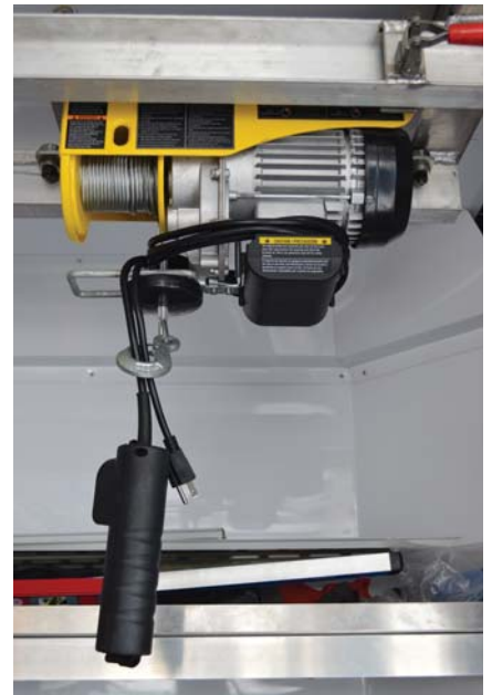
Victor developed this unique trailer hoist for handling bigger coils. They are installed in every trailer.
