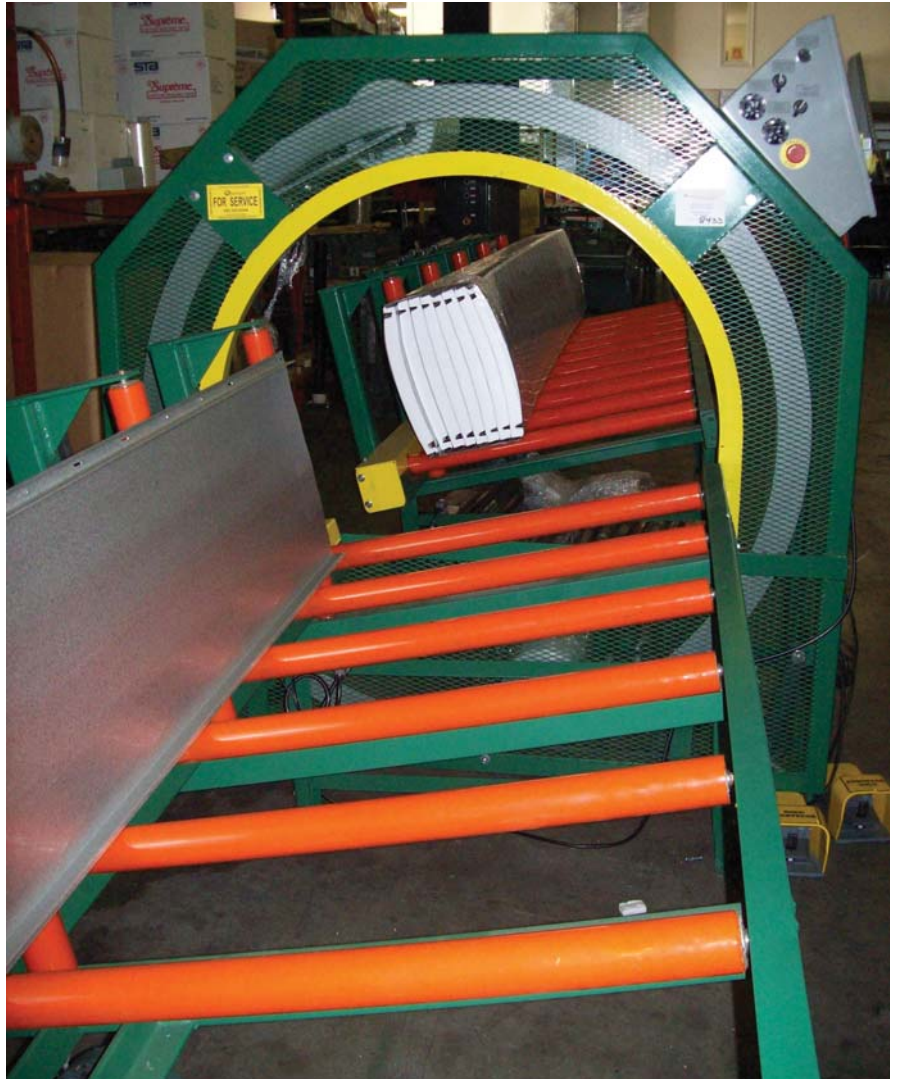
The Ameripak SR-42T series wrapper holds the integrity and finish of metal molding and trim to protect from damage in transit.
