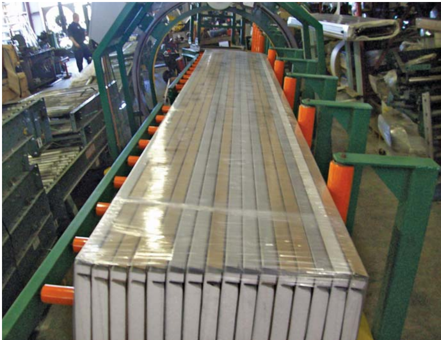
For a standing seam production line, the Ameripak SR-442SS series is designed to unitize and protect the panels to allow an increase in panel production.
