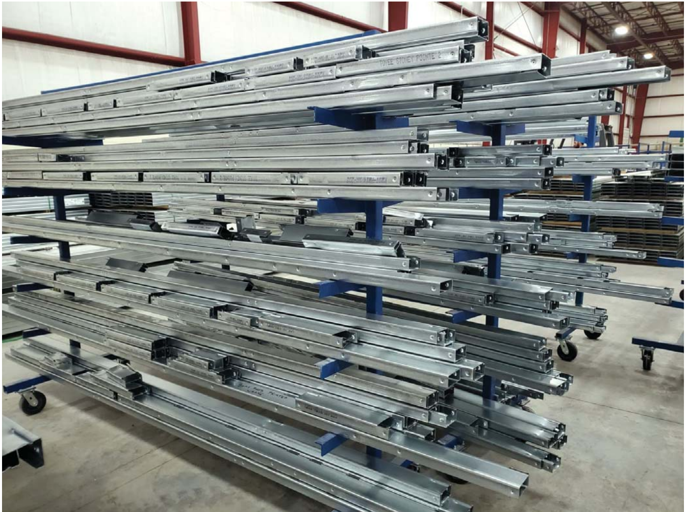
Wall studs and track ready to be assembled. Photo courtesy of ToVee
