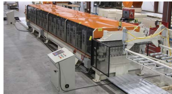
Tober uses this Howick roll-forming machine to create 16 gauge 3-5/8" studs and track for framing out of REVIT design software. Steel coil is sourced from several U.S. vendors. Photo courtesy of ToVee
