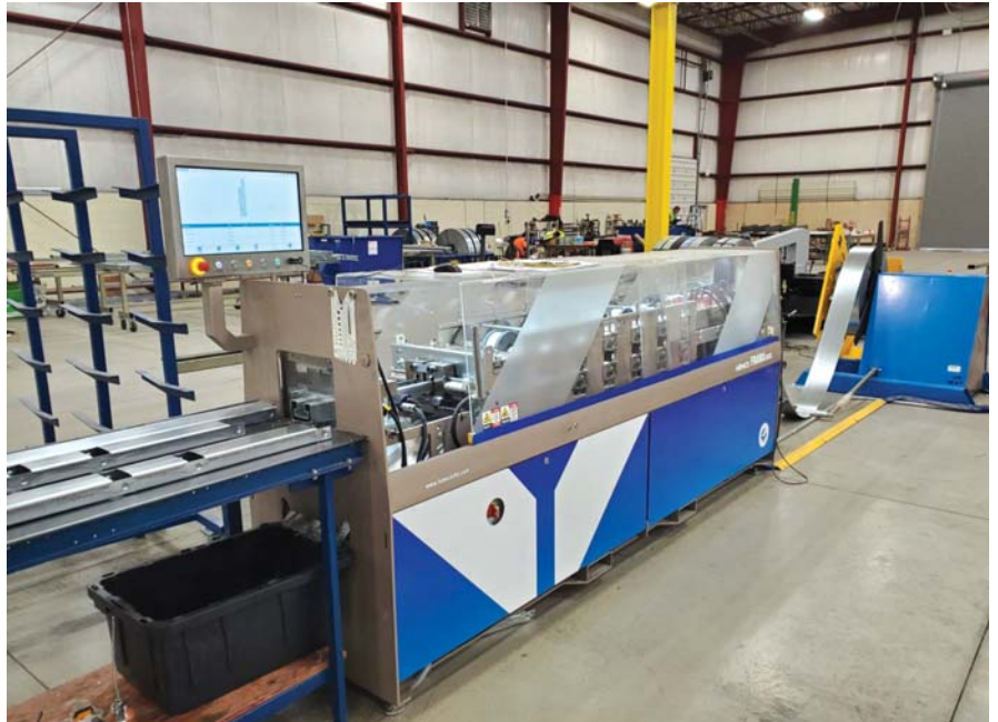
Tober uses this Howick roll-forming machine to create 16 gauge 3-5/8" studs and track for framing out of REVIT design software. Steel coil is sourced from several U.S. vendors. Photo courtesy of ToVee
