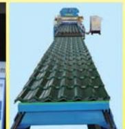
• Automatic Stacking Table & Conveyor
