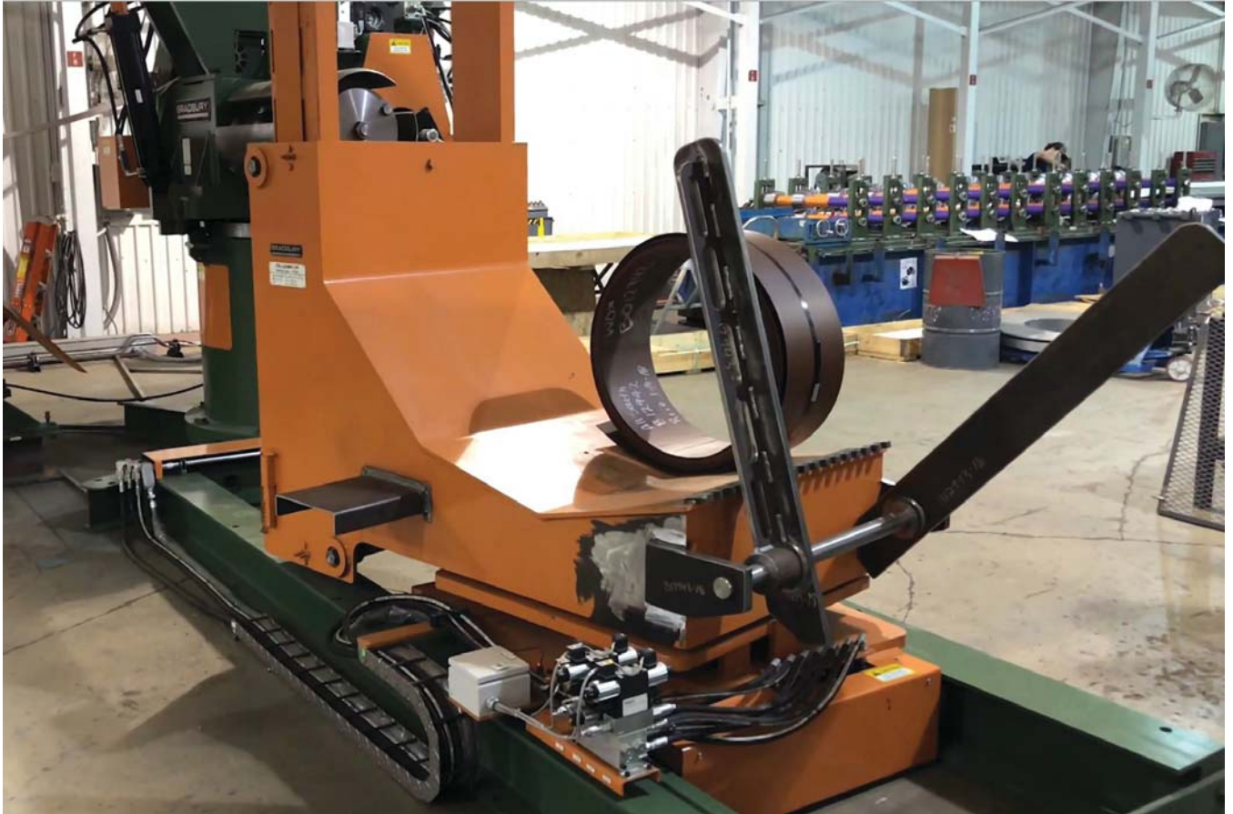
Typically, a forklift driver must approach a coil car perpendicular to line flow, but in this situation existing facility constraints offered no room for traditional maneuvers. When The Bradbury Company got the call seeking a solution, they created this custom rotating coil car. The forklift driver can now load a coil parallel to line flow. PHOTO COURTESY OF THE BRADBURY COMPANY.
