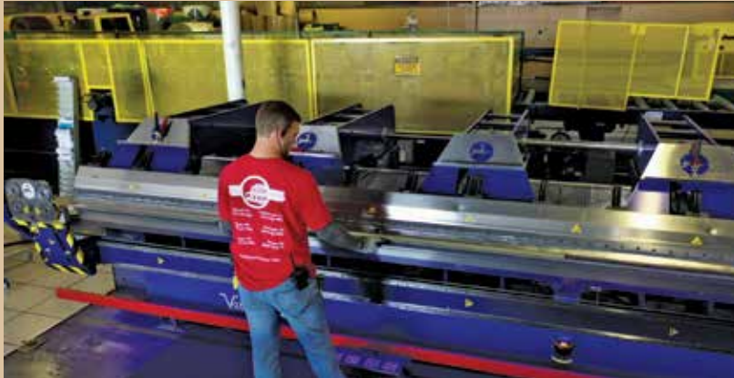
A Best Buy Metals employee works on a Variobend folder from Hershey's Metalmeister
