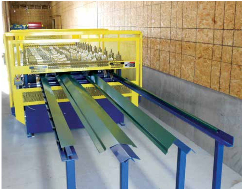
Metal Rollforming Systems designs, manufactures, and sells trim rollforming equipment that makes quick work out of all your flashing needs. With the ability to produce 700 pieces of 10' trim in an hour these machines can be tooled to make anything from corners, J channels, ridge caps, box eaves, and more.
