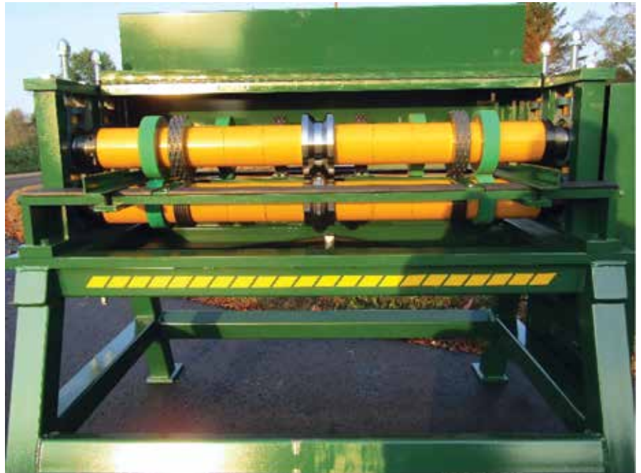
To better serve his customers by providing perforated panels and trims, Nathan Yoder ordered a new perforator machine from Acu-Form, with which he will be able to make soffit and other ventilated panels. PHOTOS COURTESY OF ACU-FORM
