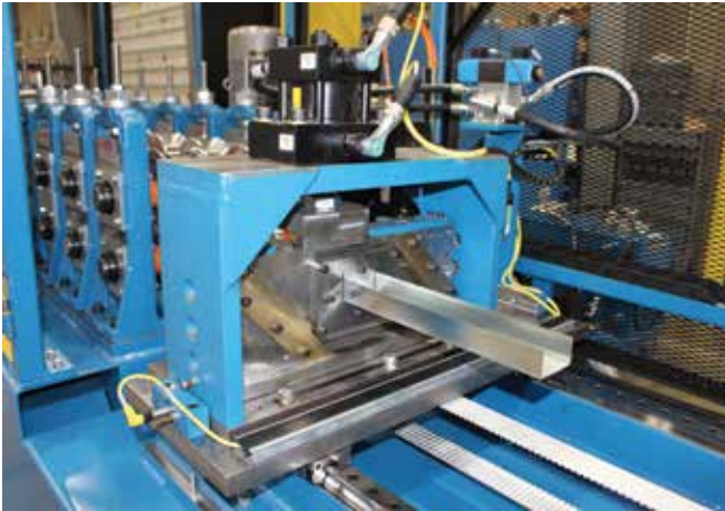
(LEFT) An ASC Machine roll-forming machine produces U channel, which is used for framing. PHOTO COURTESY OF ASC MACHINE TOOLS
