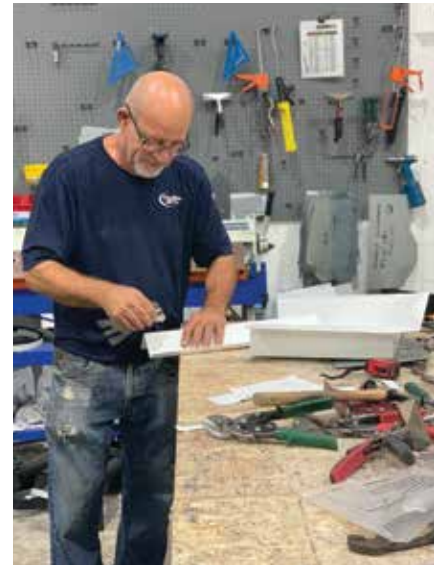
Carlos, one of the Coastal Metals metal sheet fabricators, handcrafts a chimney cap at the company's warehouse in Miami. PHOTOS COURTESY COASTAL METAL ROOFING SALES.
