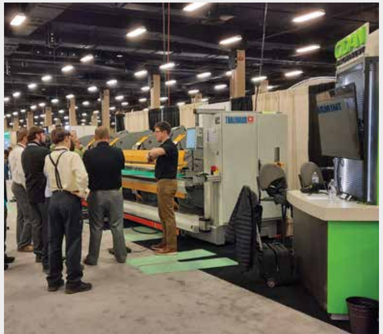
Positioned right inside the entry, CIDAN Machinery exhibited a Thalmann TD150 Double Folder. It folds the material both up and down, which minimizes operator intervention. Find CIDAN at the Construction Rollforming Show in October.
