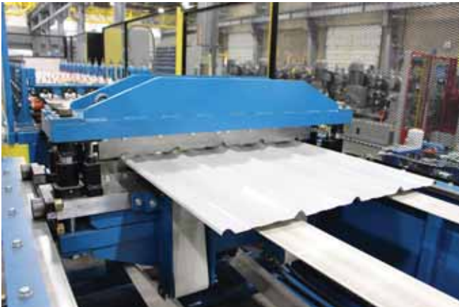
End flare should be minimal on a good quality post-cut machine. PHOTO COURTESY OF ASC MACHINE TOOLS
