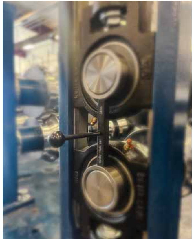
With the help of a gauge block, users can reset their roll forming machine to factory zero. PHOTO COURTESY OF METAL ROLLFORMING SYSTEMS.
