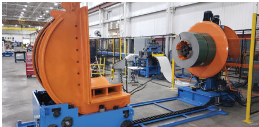
A coil car and upender combo allows for a coil to be loaded on the coil car while the uncoiler is still running.
