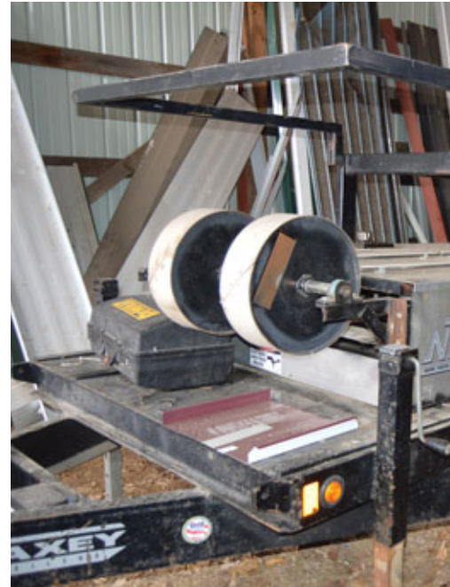
Luke Herschberger purchased a used New Tech Machinery portable roll former in his roofing business before founding Mapleview Metal Forming.
