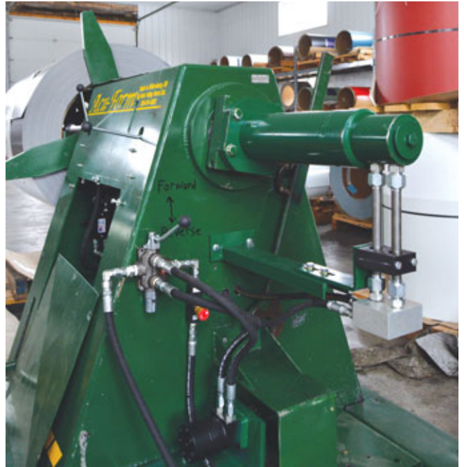
The Acu-Form decoiler was recently converted from mechanical to hydraulic, which has reduced the noise and fumes in the shop.
