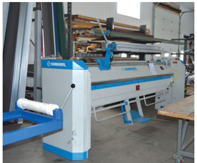
The Schechtel trim brake is critical for making trim. PHOTOS BY KAREN KNAPSTEIN
