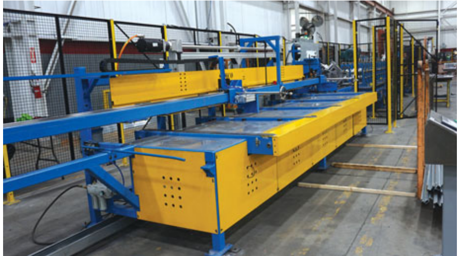
A nester eliminates the need for multiple workers at the end of the roll forming line.
