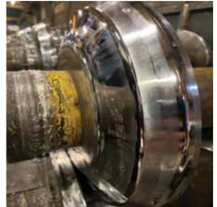
Worn tooling typically occurs gradually over time and is not always recognized immediately by the daily machine operator. PHOTO COURTESY OF THE BRADBURY GROUP.
