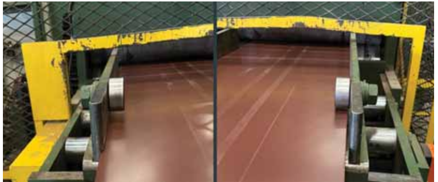
Problems can arise at lead-in or entry guides showing up as inconsistent width entry and exit. When caught early, small adjustments can avoid damage to panel and machine. PHOTO COURTESY OF THE BRADBURY GROUP.
