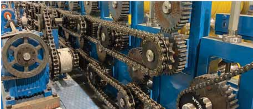
Maintaining proper lubrication is essential for the longevity of your roll former. This includes inspection of bearings, bushings, gear boxes, chains, sprockets, and spur gears. PHOTO COURTESY OF THE BRADBURY GROUP.
