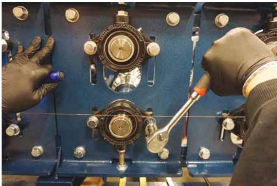
Vibration from normal use can loosen bolts. Inspect machines before and during operation so little things like this don't turn into big headaches. PHOTO COURTESY OF METAL ROLLFORMING SYSTEMS
