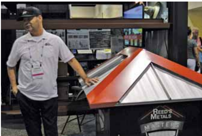
Jasson Johnson, trainer in Reed's Metals' Masters program, explains how the stations are used in the training program. The components in red are the pieces that students learn to form at this particular station.
