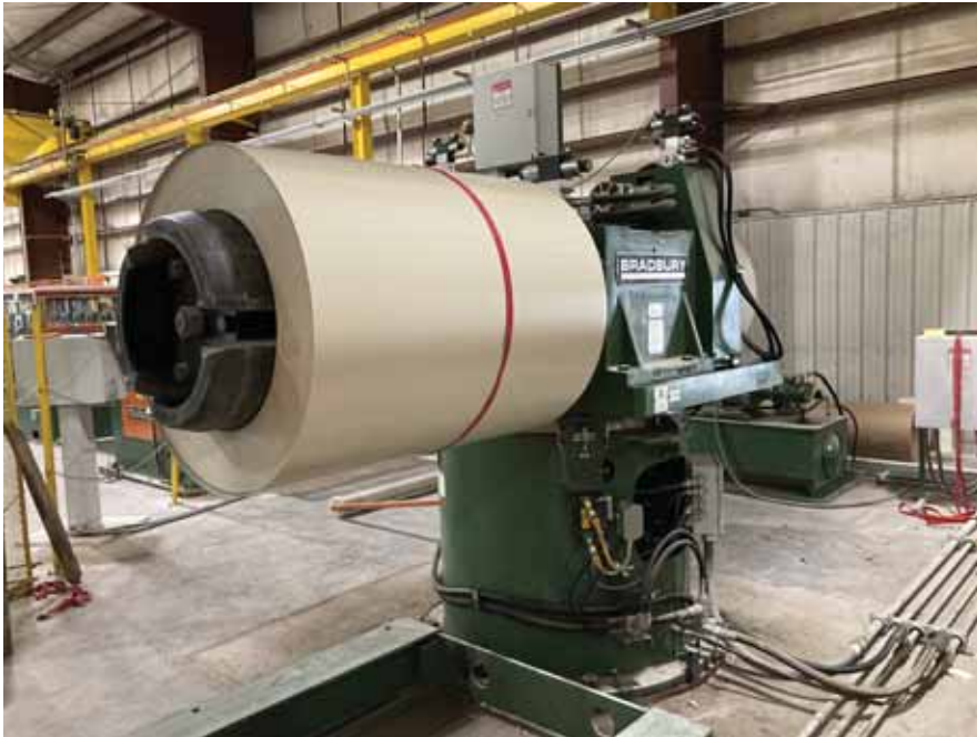
Double mandrel uncoiler easily handles 15,000-pound coils.
