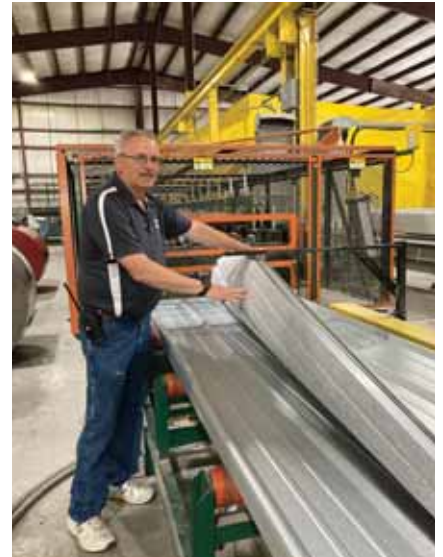
Owner Dave Higgins showing the underside of a DripStop-coated panel.
