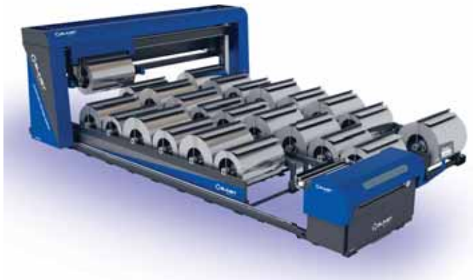
A high quality gang slitter cuts all the pieces from the flat stock at once, reducing the risk of bow and taper. Above: The Slinet from Hershey's Metal Meister.
