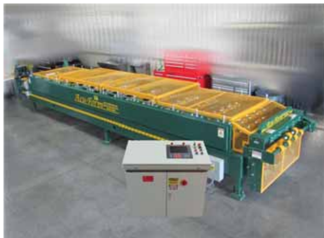
Every fraction of an inch counts when rolling steel. To avoid any waste, Acu-Form offers servo drive controls that can assure no more than a 1/32 of an inch cutting variable. ACU-FORM PHOTO
