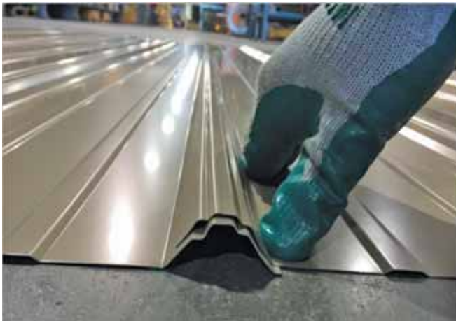
A loose overlap between two connecting panels resulting from wavy edges can result in installation and performance issues. BRADBURY PHOTO
