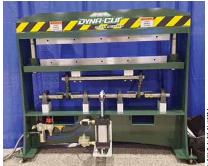
PHOTO BY KAREN KNAPSTEIN ABOVE: The Dyna-Cut Metal Muncher ready for blades custom made to fit the panel profile. BELOW: With custom blades installed.
