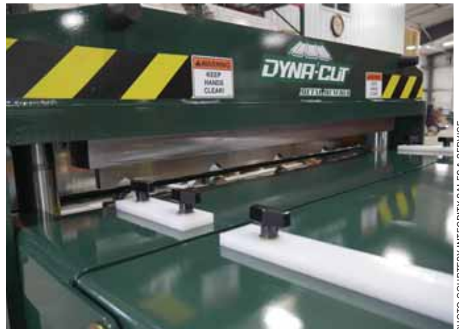
PHOTO BY KAREN KNAPSTEIN ABOVE: The Dyna-Cut Metal Muncher ready for blades custom made to fit the panel profile. BELOW: With custom blades installed.
