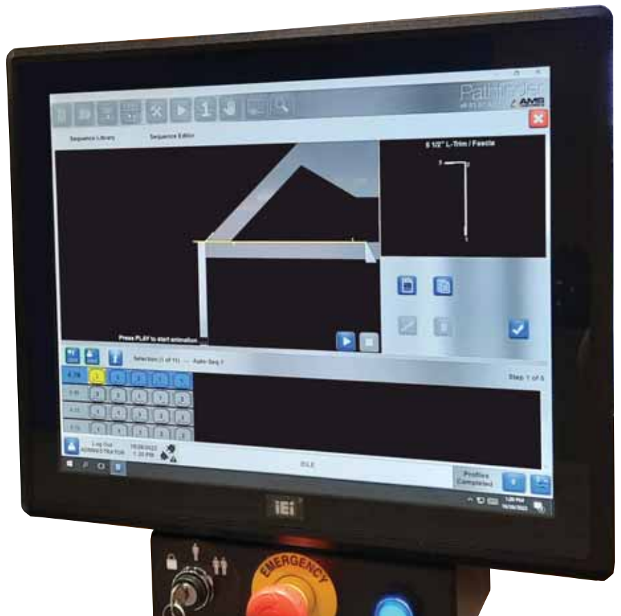
Auto sequencing tools help identify bend sequences efficiently. PHOTO COURTESY OF AMS CONTROLS
