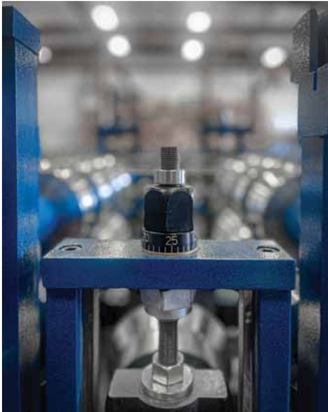
A minimum clearance positive stop device on calibration nuts for MRS machines is helping operators avoid adjustment errors. MRS PHOTO
