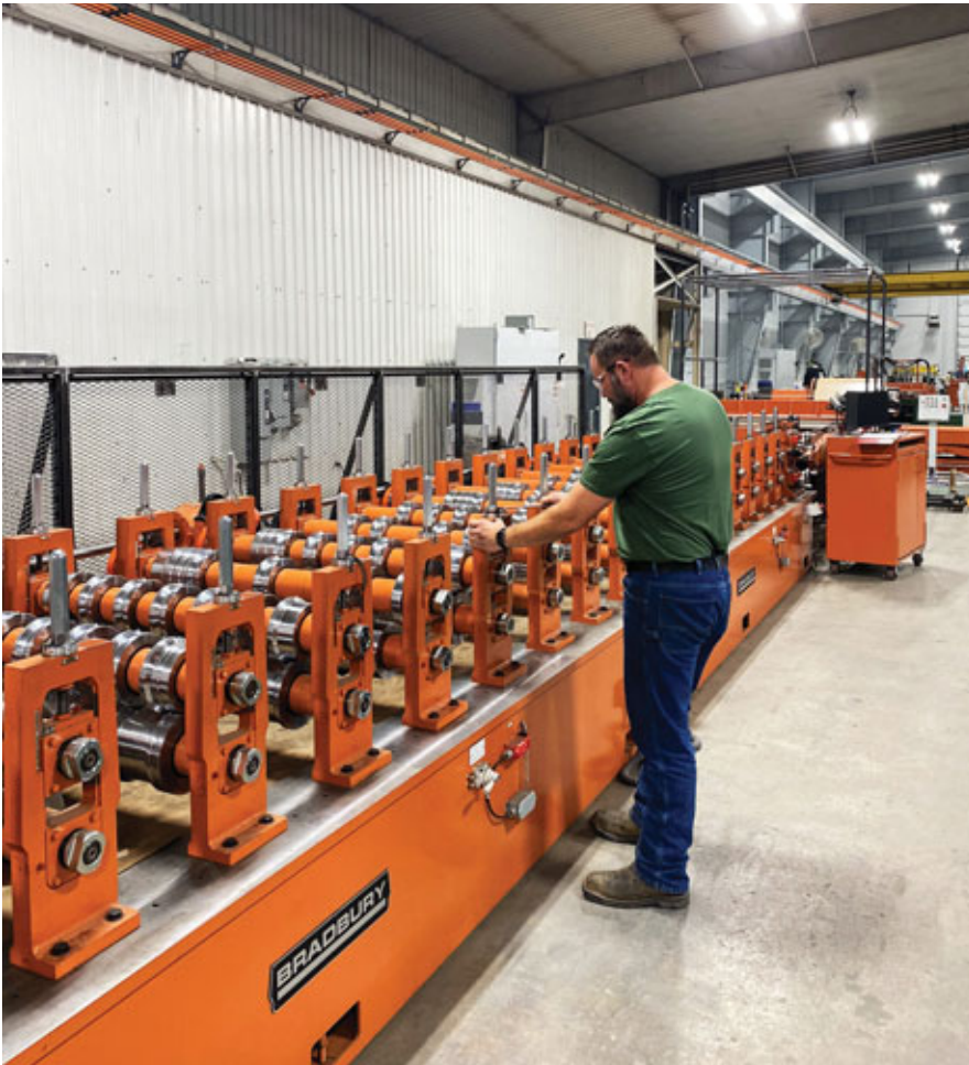
A roll forming line requires a space of approximately 90 feet long by 10 feet wide to operate safely.
