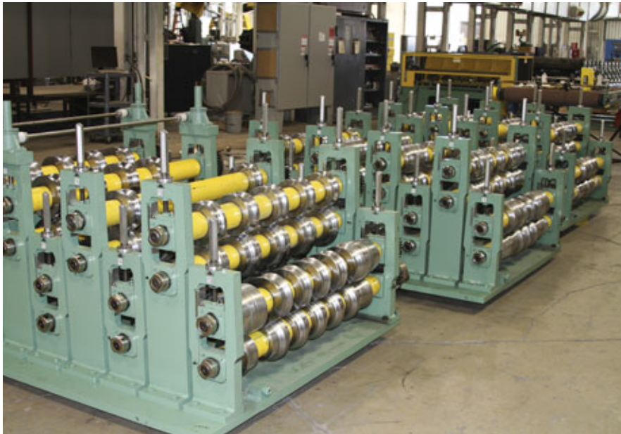
Bradbury tooling rafts for rafted roll former. A rafting roll former allows you to interchange tooling for each profile. Photos courtesy of The Bradbury Group.
