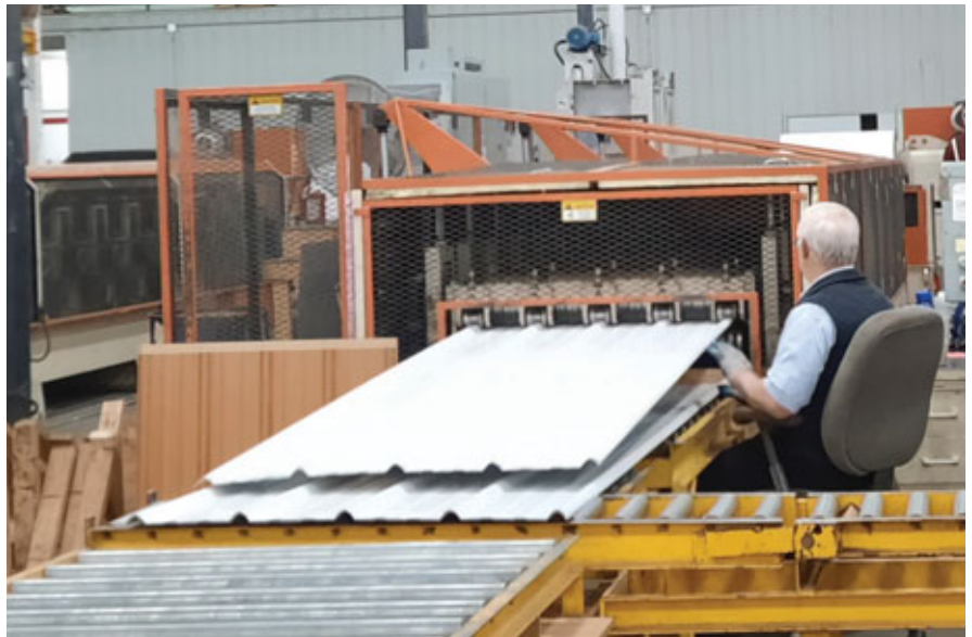
Protect your dies and your panels. If running thicker material, you may need to back off the die position. PHOTO BY SHIELD WALL MEDIA.
