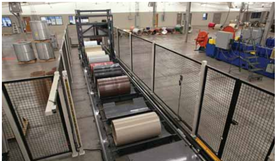
A better look at the 12-station CX-5 coil changing system installed at American Building Network (Central Steel Group), Mount Airy, North Carolina.
