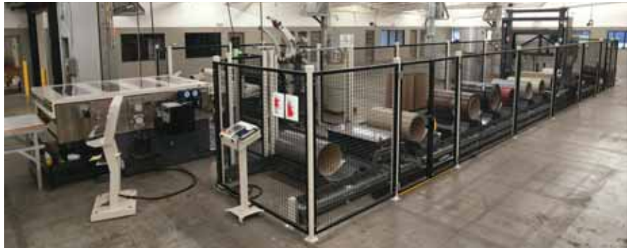
Guards surround the coil farm, preventing injury to workers and damage from equipment moving around the floor. ALL PHOTOS COURTESY OF CENTRAL STEEL GROUP MARKETING.
