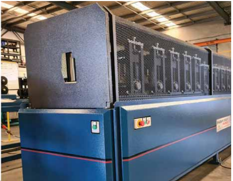
The Bradbury Sculptured Gutter Machine is a shop-based machine that is used by high-volume suppliers in the metal building industry. PHOTO BY BRADBURY CO.
