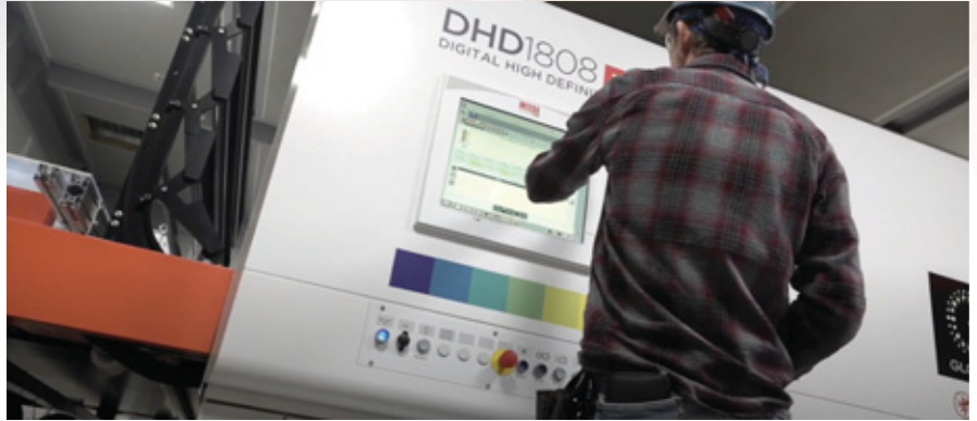
400 DPI scans create realistic images of wood that can be manipulated to add additional elements prior to being transferred to metal. SDI PHOTO
