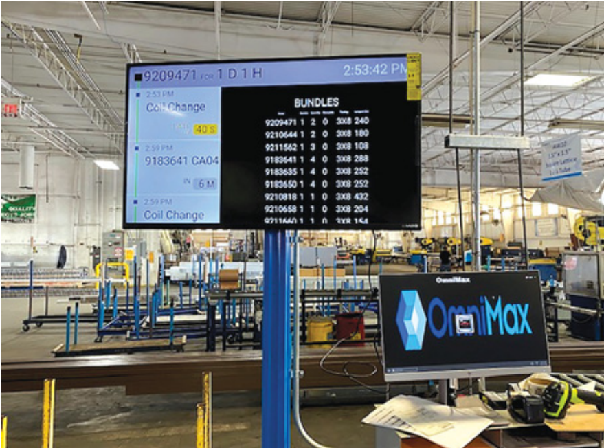
Andon boards are a simple way to help keep employees on task and informed of job progress. AMS CONTROLS PHOTO
