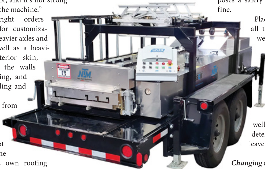
A Maxey open-bed trailer mounted with a New Tech SSQII roof panel machine. NEW TECH MACHINERY PHOTO.
