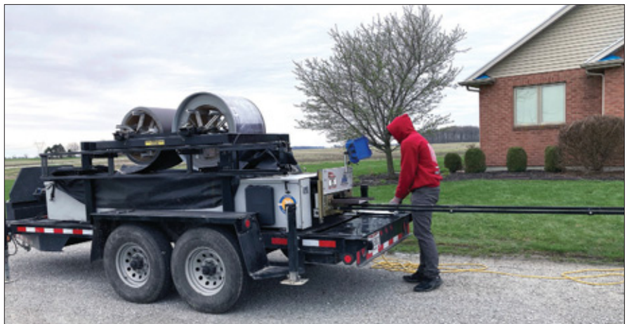
Panels being formed on a New Tech SSR portable roll former.
