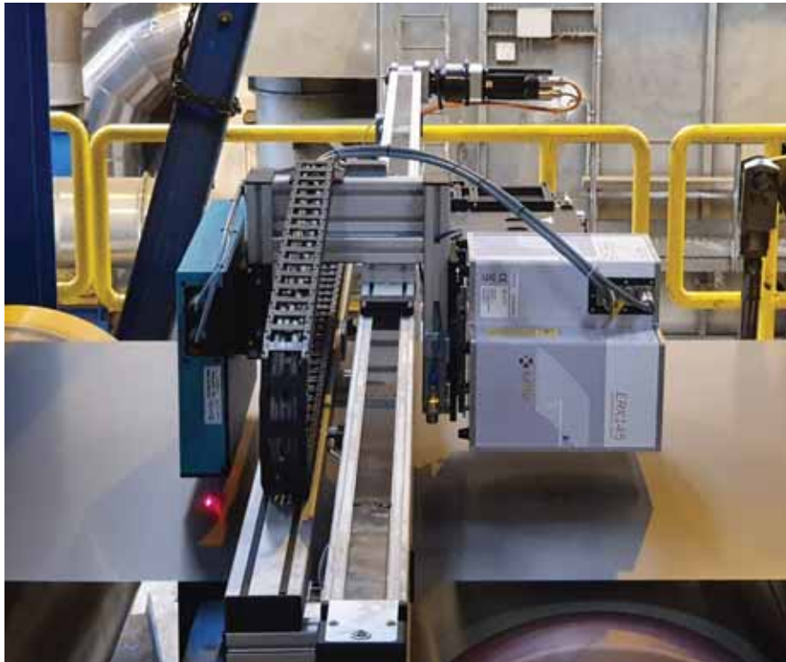
Measuring color on hot coated surfaces. Inline devices, like the X-Rite ERX145, have a built-in pyrometer to measure the current temperature of the coil right at the measurement spot.
