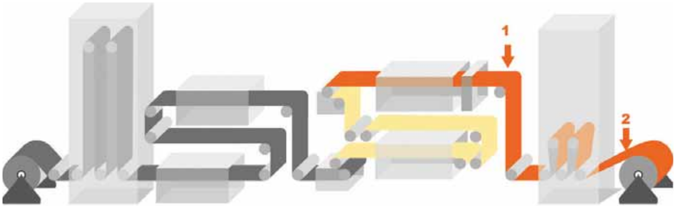
Measurement positions at the coil coating machine. 1) After water quench. 2) Before reel up.
