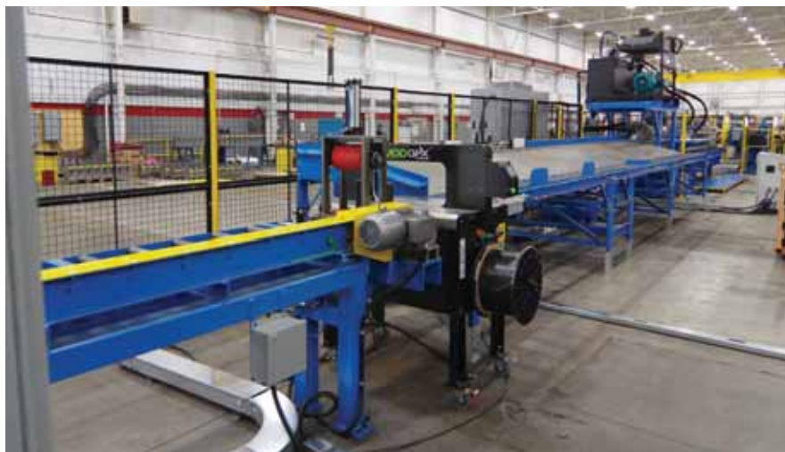
Bundlers automate the handling of mini-bundles and automatically build pre-programmed master bundles ready to be shipped based on orders.
