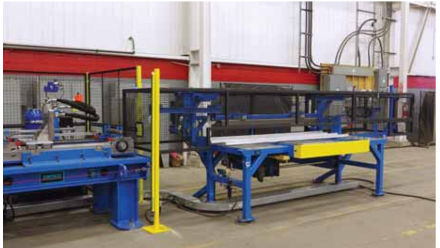
A nester collects and nests a bundle of finished products and sets them up for shipping.
