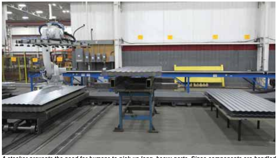
A stacker prevents the need for humans to pick up long, heavy parts. Since components are handled by machines, it's less hazardous for humans.
