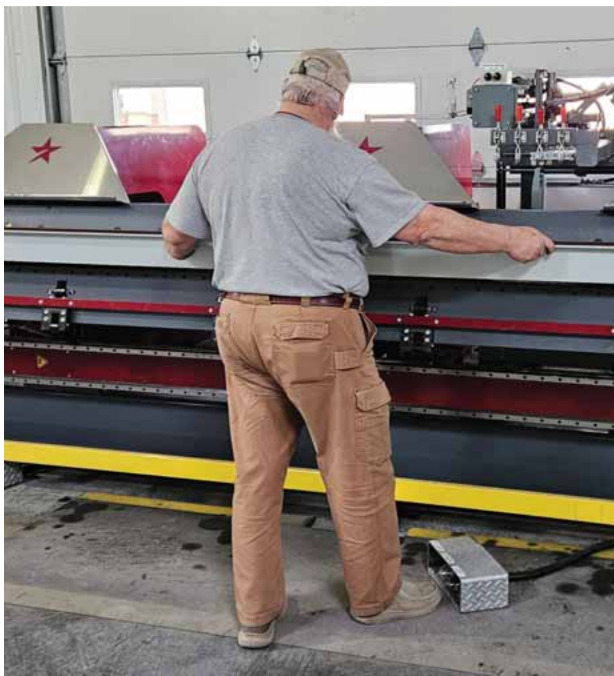
Operation is simple: Insert the template. Use the down pedal to clamp the work piece, and press start to bend. The up pedal is used to open the clamp, if needed. PHOTOS COURTESY OF STAR 1 PRODUCTS.
