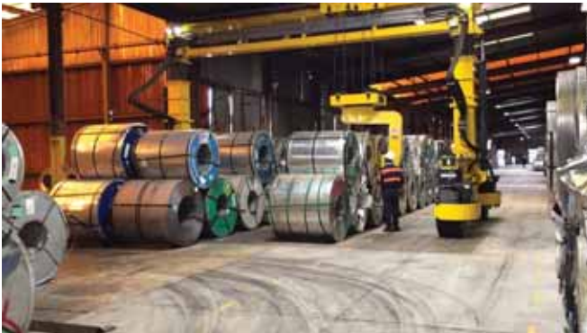
Combi-MG equipped with a rotating C-hook for handling coils and operated by remote control.
