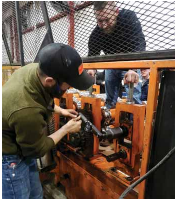
Any regular maintenance on your roll former should include the alignment of critical components. PHOTO COURTESY OF THE BRADBURY GROUP
