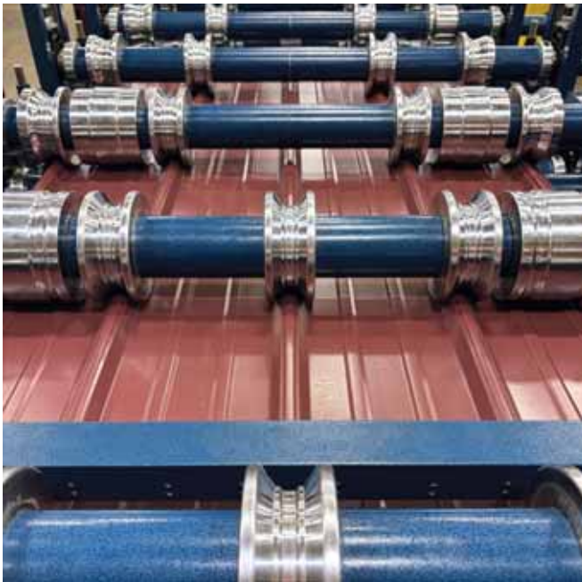
Tooling must be kept clean because it creates the product that heads out the door to the customer. PHOTO COURTESY OF METAL ROLLFORMING SYSTEMS.
