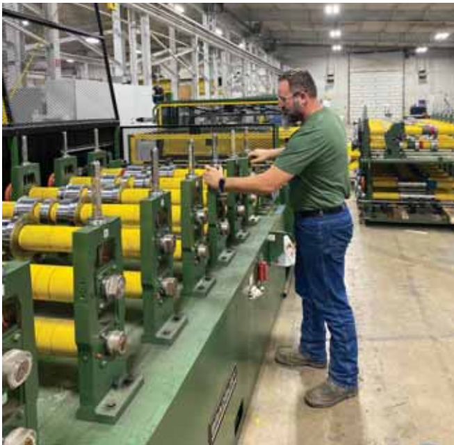
If your roll former is not producing consistent product, the problem can be remedied by adjusting the roll tooling. PHOTO COURTESY OF THE BRADBURY GROUP
