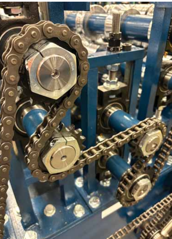
Improperly tensioned chains have the potential of causing a lot of premature wear and damage. PHOTO COURTESY OF METAL ROLLFORMING SYSTEMS.
