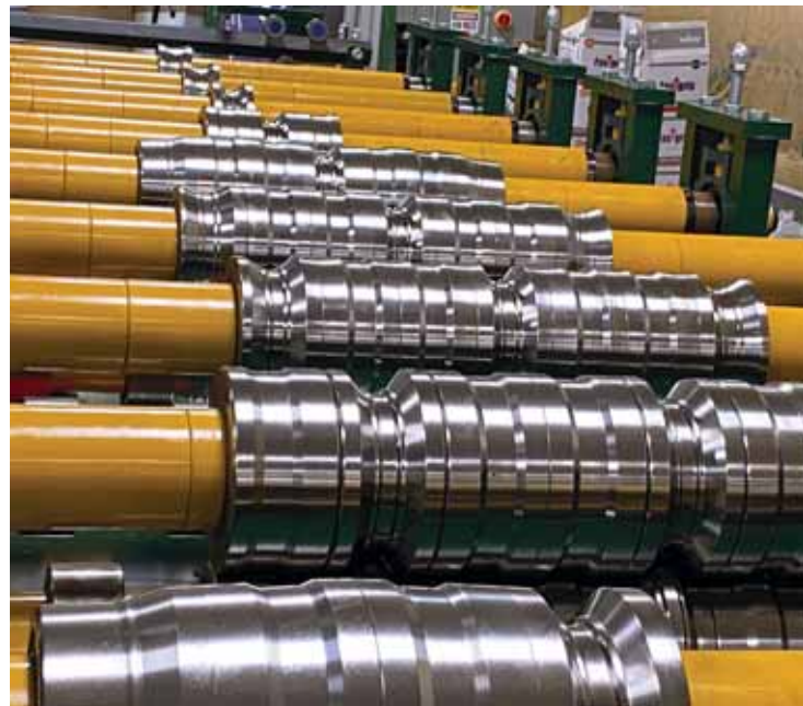
Clean tooling and forming surfaces are important for producing consistent product quality. PHOTO COURTESY OF ACU-FORM.
