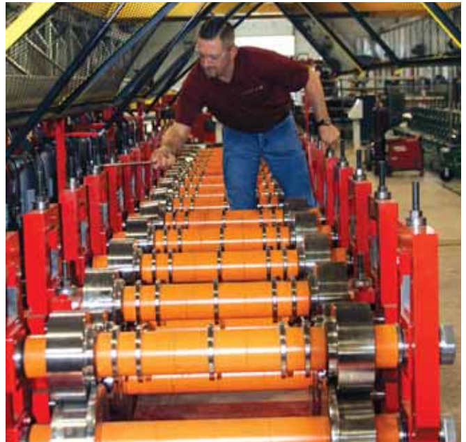
You want your roll former to produce consistent product, so it's important to inspect and calibrate the machine's tooling.
