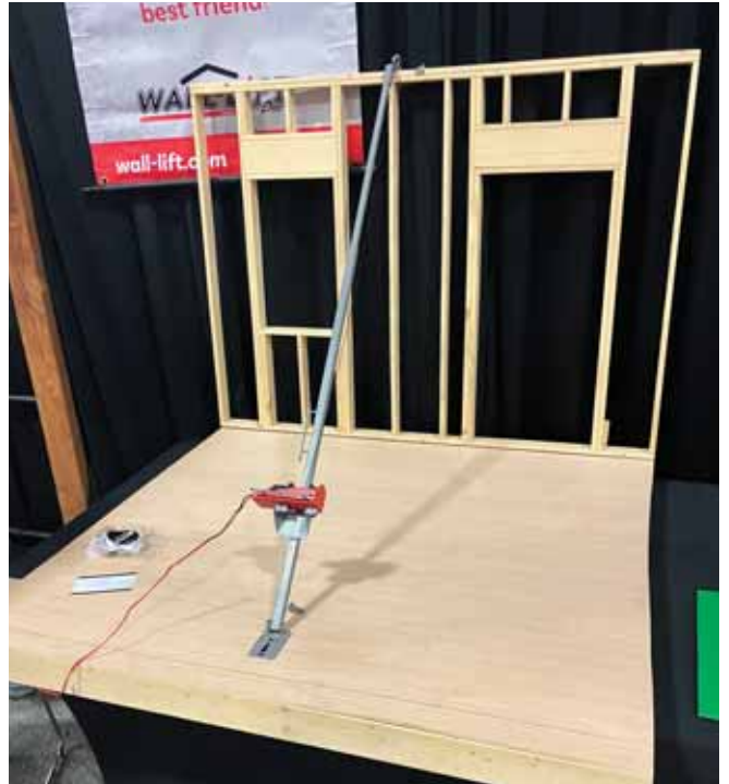
Wall-Lift is a powered hoist system for lifting walls. Each unit can lift 440 pounds. A small but powered demonstration unit was on display.
