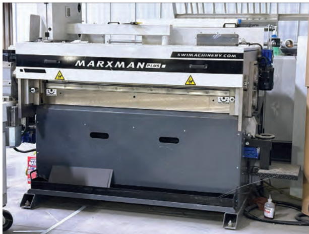
The Marxman Plus slitter and Variobend folder are used to produce metal trims for roofers. SHIELD WALL MEDIA PHOTOS.
