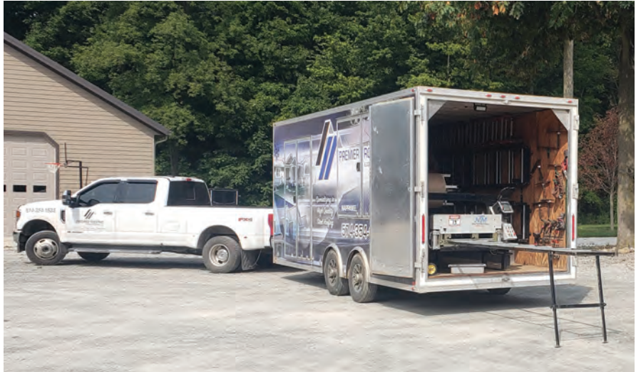
Each portable trailer is a fully autonomous unit, complete with all supplies necessary to complete the job and a power unit. Photos courtesy of Premier Roofing & Construction unless otherwise indicated.
