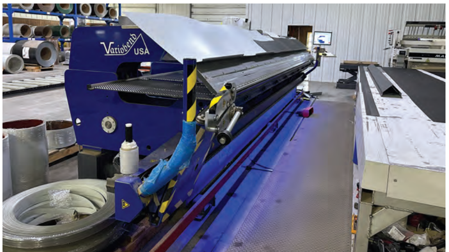
The Marxman Plus slitter and Variobend folder are used to produce metal trims for roofers. SHIELD WALL MEDIA PHOTOS.
