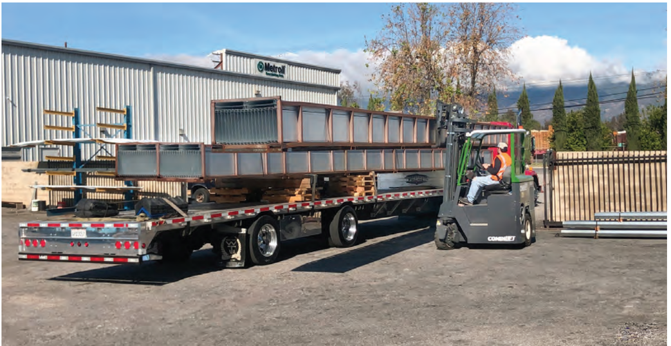
Metroll-Southern California, using Multidirectional Combilifts to load 30-ft. roll-formed cladding onto trucks. PHOTO COURTESY OF COMBILIFT.
