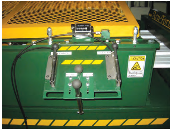
In a mechanical setup, levers operate the panel direction and shear. PHOTO COURTESY OF ACU-FORM
