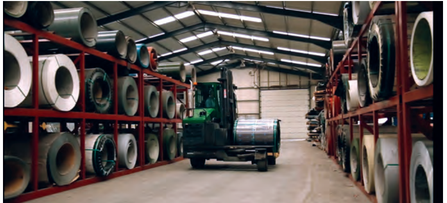
If weight is distributed evenly over the wheels, the result is better load stability. PHOTO COURTESY OF COMBILIFT.
