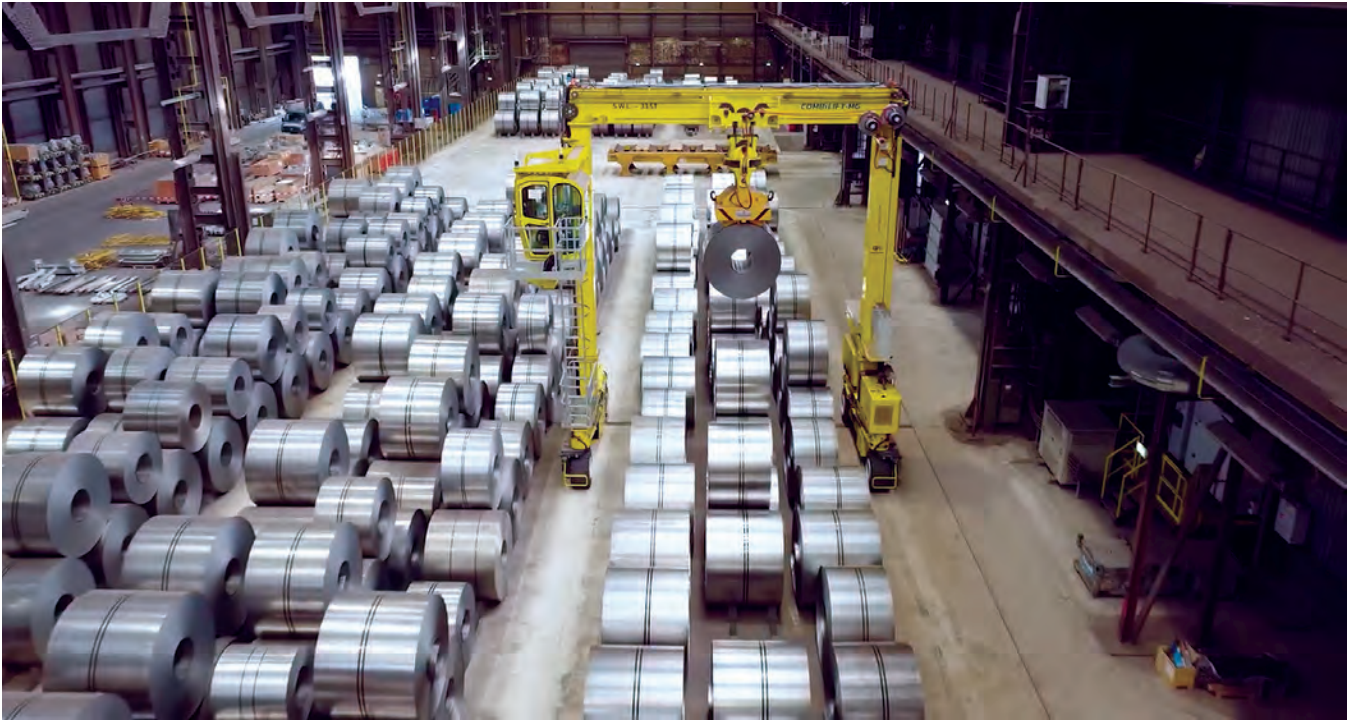
Minimizing the number of times a coil is handled also minimizes the risk of damage and injury. PHOTO COURTESY OF COMBILIFT.
