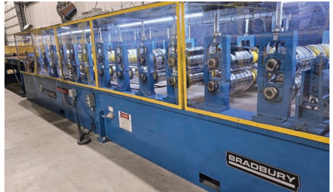
One of Ramco's high-speed Bradbury roll forming lines.
