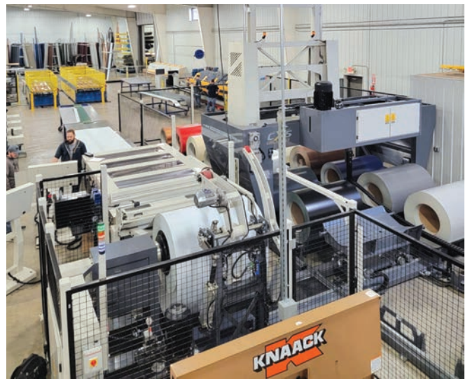
This recently installed SWI CX5 Coil XPress is paired with the SWI Marxman PRO, allowing for efficient coil change-outs through an integrated coil management and slitting operation. PHOTO COURTESY OF SWI MACHINERY
