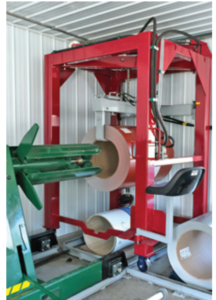
The position of the operator gives them a better view throughout the coil picking and moving process. PHOTOS COURTESY OF STAR 1 PRODUCTS.
