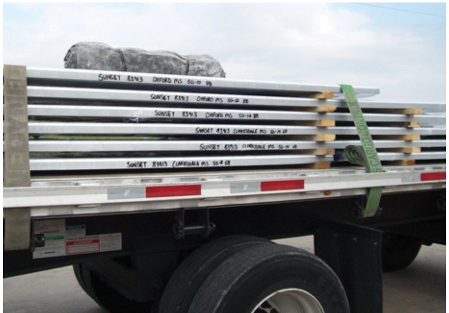
This manufacturer writes order information in permanent marker directly on shrink wrap. PHOTO COURTESY OF AMERIPAK, INC.
