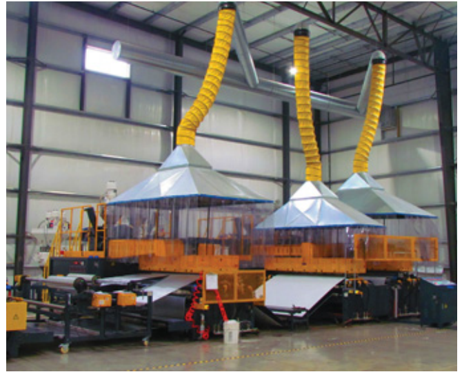
Safety measures for MWI Components' reflective insulation machine include high-visibility caution tape on the floor, extensive machine guards, cautionary paint, and air pollution mitigation.
