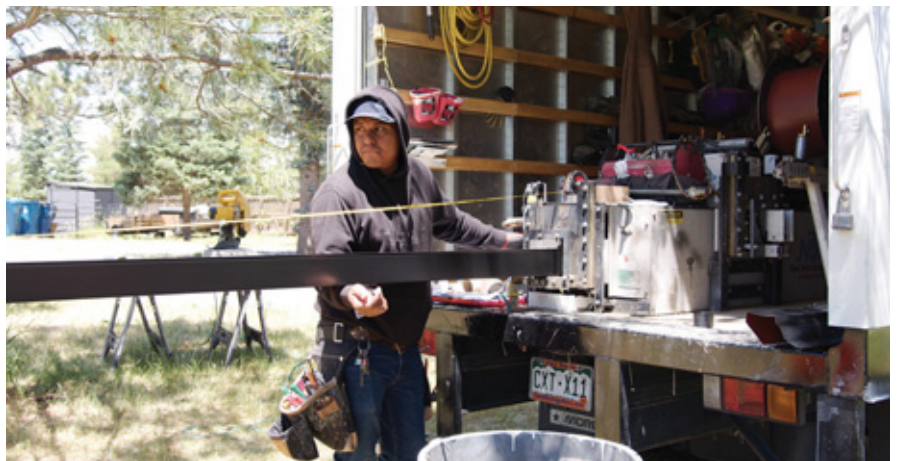
Roll forming rain gutters with a New Tech machine.
