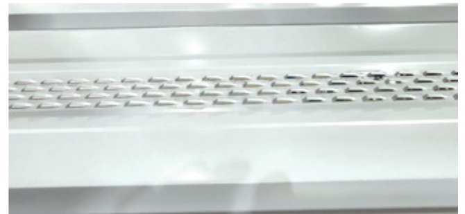
A clear view of the back side of a perforated panel. PHOTO COURTESY OF ROLL FORMER LLC.
