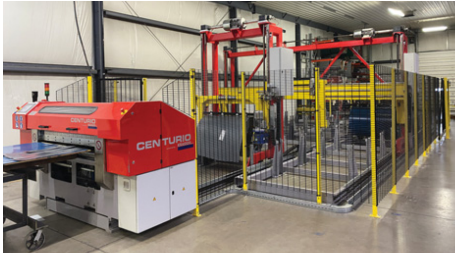
Safety guards should remain in place unless equipment is locked out and tagged out. PHOTOS COURTESY OF MWI COMPONENTS
