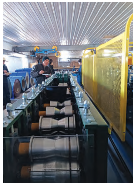
Attendees could get an up-close look at the new roll forming shop equipment while enjoying a hog roast with all the trimmings. Shown here: An Acu-Form mechanically powered roll former for making F and J trim.
