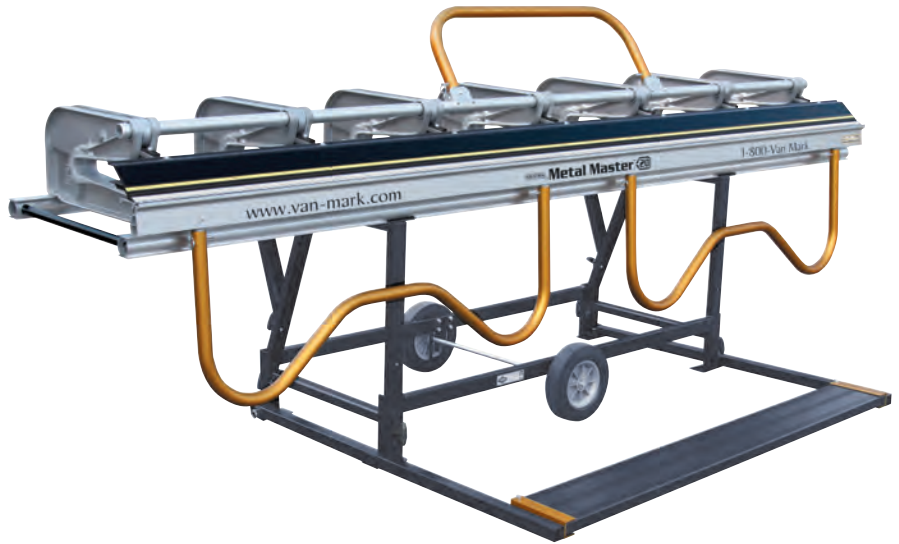
The Van Mark Industrial Metal Master 20 manual brake comes with a stand and platform that enables users to increase leverage and stabilize the brake while working with heavy materials. PHOTO COURTESY OF VAN MARK
