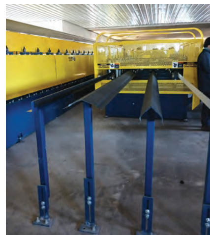
The MRS trim machine makes four different components: J channel, ridge cap, big corners, and little corners.
