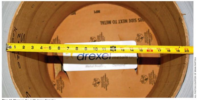
Step #1: Measure the coil's inner diameter.
