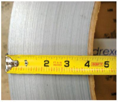
Step #2: Measure the material's thickness on one side of the coil.
