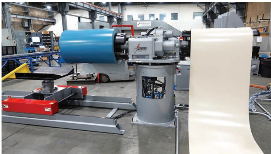
ASC Machine Tools double-arm uncoiler, 10,000 pound capacity, with coil car. COURTESY OF ASC MACHINE TOOLS.
