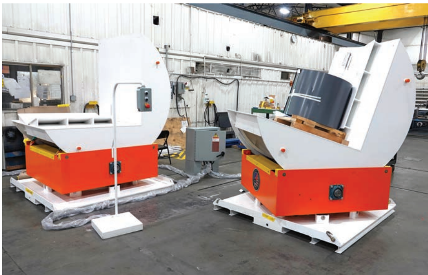
ASC Machine Tools rotating upender. COURTESY OF ASC MACHINE TOOLS.
