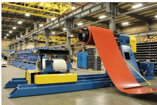
ASC Machine Tools single-arm uncoiler with coil car. COURTESY OF ASC MACHINE TOOLS.
