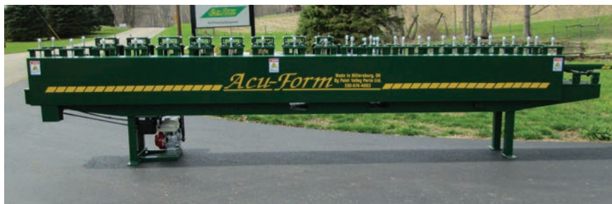
The amount of tooling required has a significant impact on the price of the machine. A basic profile like a ridge cap requires only 10 stands, while an F & J channel machine needs more tooling. PHOTOS COURTESY OF ACU-FORM EQUIPMENT.
