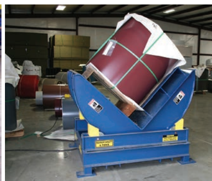
MRS single-station uncoiler (left) and upender (right). COURTESY OF METAL ROLLFORMING SYSTEMS.
