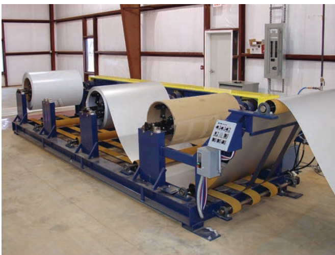
Metal Rollforming Systems multi-station decoiler. COURTESY OF METAL ROLLFORMING SYSTEMS.
