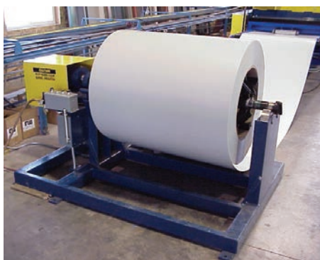
MRS single-station uncoiler (left) and upender (right). COURTESY OF METAL ROLLFORMING SYSTEMS.
