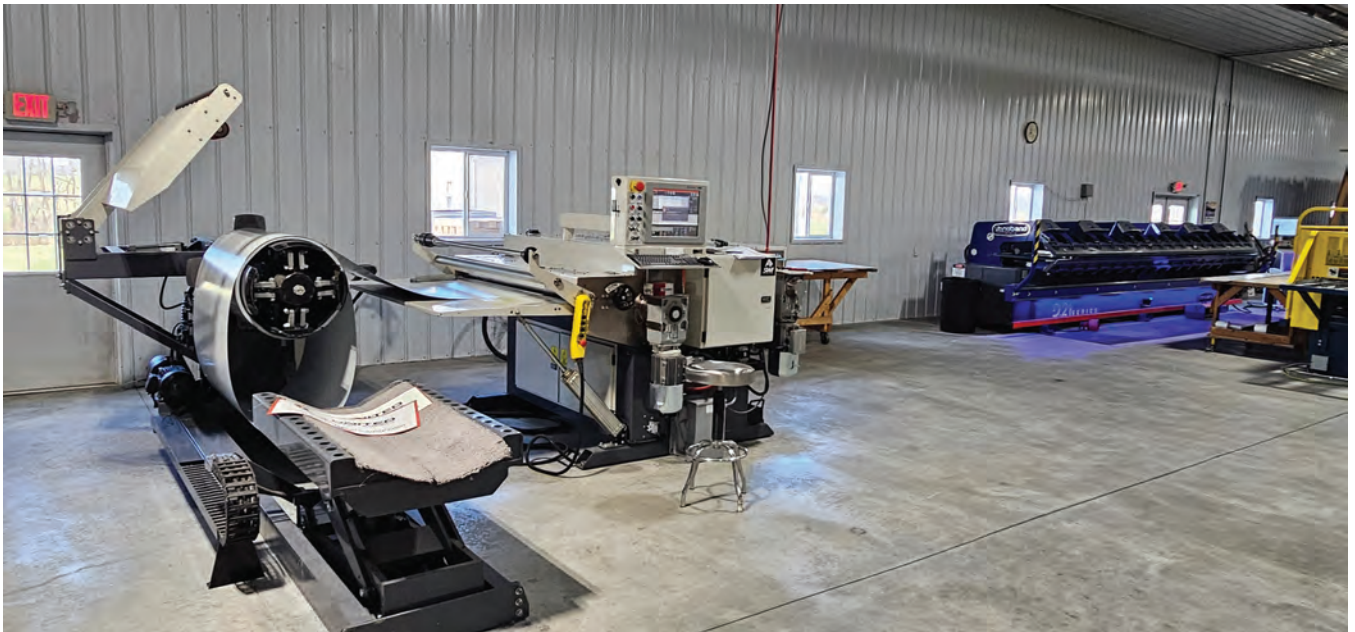
The Marxman slitting line from SWI Machinery (above left), and the Variobend double folder stand at the ready.
