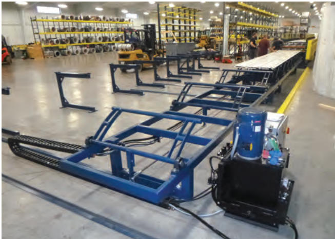
Exit or runout table. PHOTO COURTESY OF METAL ROLLFORMING SYSTEMS
