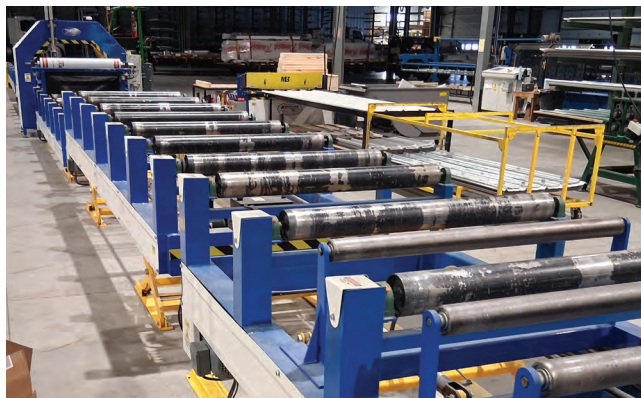
Power Lift & Roll Table for dual deck roll former. PHOTO COURTESY OF HEARTLAND SALES AND MACHINE, LLC
