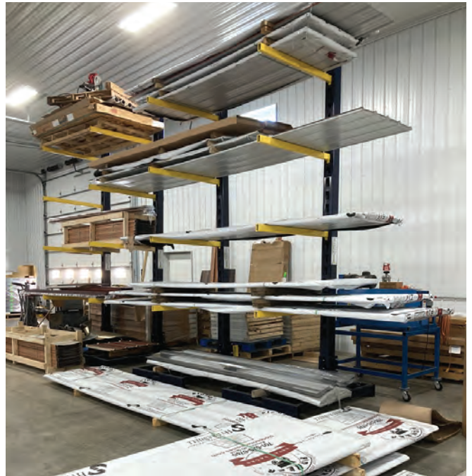
Cantilever racking. PHOTO COURTESY OF DA HOCHSTETLER & SONS
