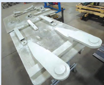
Parts are completely disassembled and restored to new condition during the Roper Whitney remanufacturing process. PHOTOS COURTESY OF ROPER WHITNEY.
