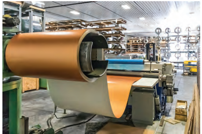
View of precision rollforming in workshop. COURTESY OF PARAGON COMPUTING SOLUTIONS
