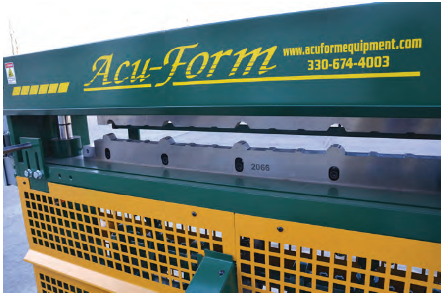
An up-close look at an Acu-Form post-cut shear. COURTESY OF ACU-FORM.
