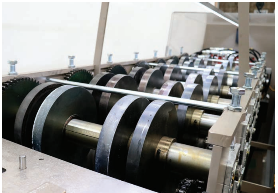
The compact design layout produces frames, trusses, panels in 3" to 8" (75 to 200mm) sections. PHOTO COURTESY OF HOWICK LTD.
