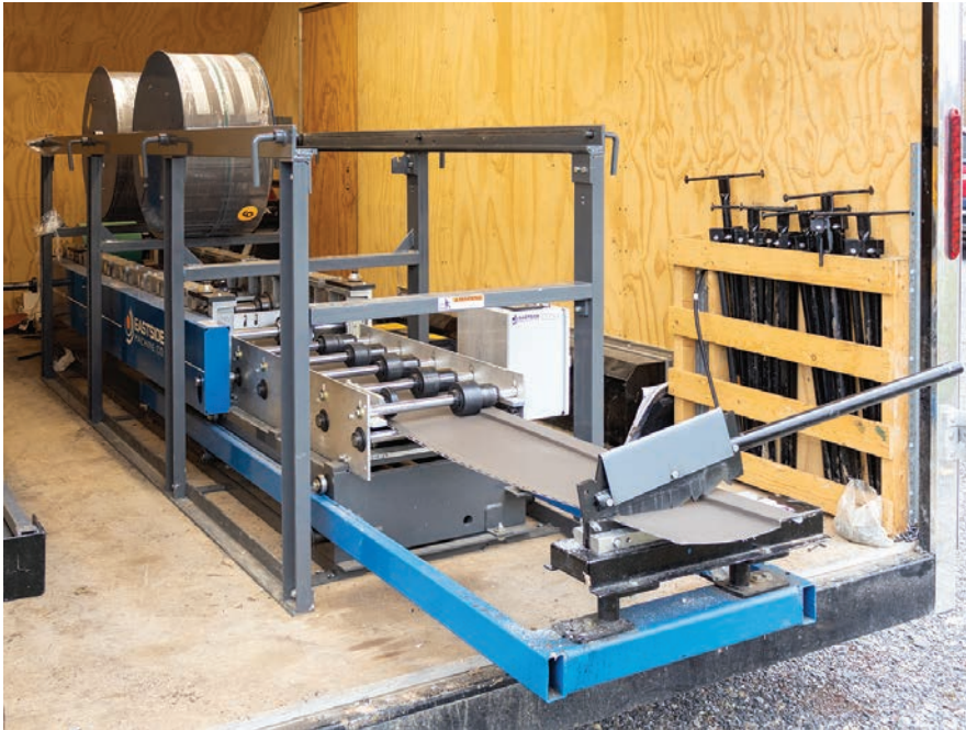
East Side Machine Board & Batten Machine.
