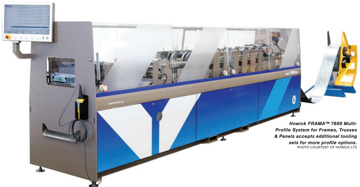
This design overcomes many traditional issues with adjustable tooling. True load-bearing frames offer cleaner structural intersections in a product range of 20 to 16 gauge (0.95 to 1.55mm). 1.55mm). PHOTO COURTESY OF HOWICK LTD.
