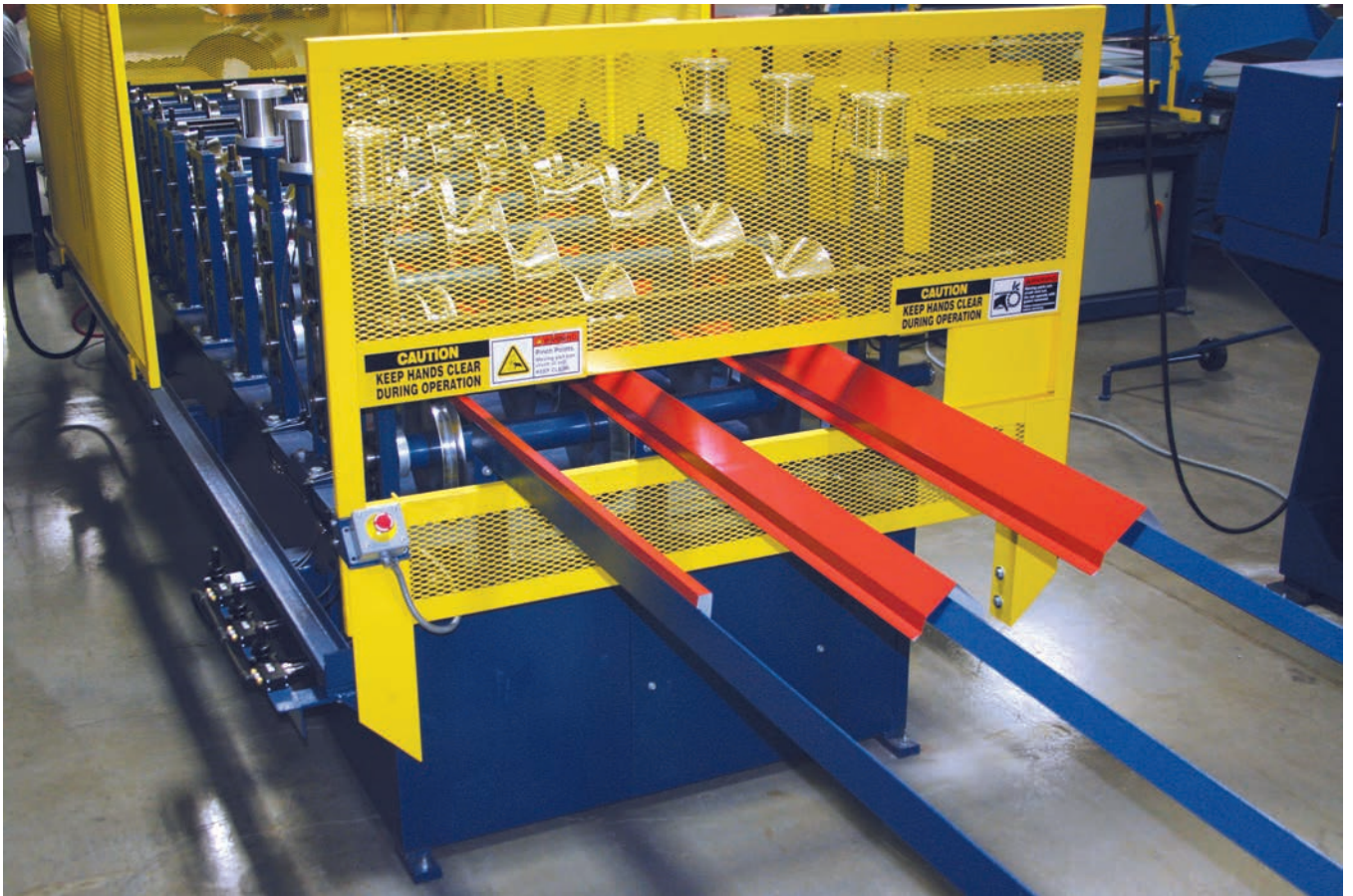
A multiple-profile roll former. When multiple tooling sets are available in the same footprint, it reduces the need for separate machines and saves space on the shop floor. PHOTO COURTESY OF METAL ROLLFORMING SYSTEMS
