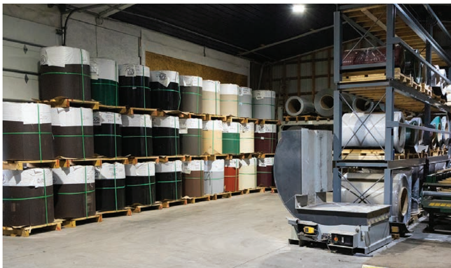
Stock painted coils from Hixwood, and an spender from Stoll Metal Works.
