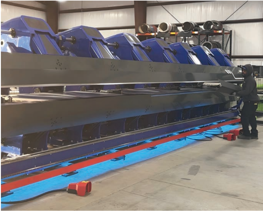
Best Buy Metals' newest 28' brake - one of its largest equipment upgrades for 2026. Operating above and beyond the standard 10'-20' capacity and enabling faster production, longer material runs, greater precision, and improved efficiency in custom panels and trim fabrication.
