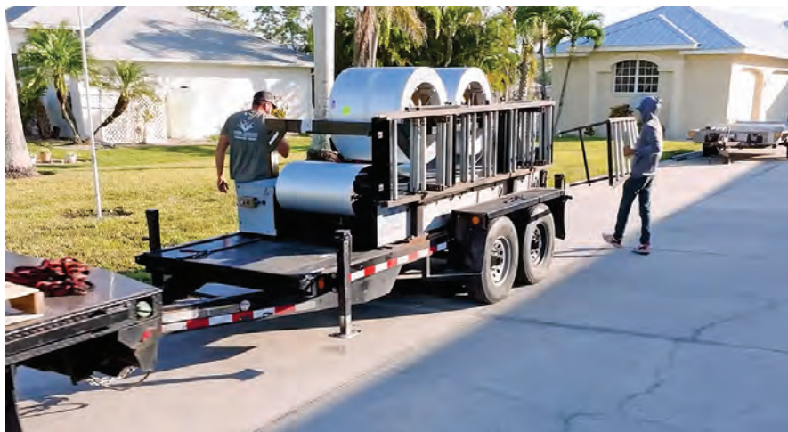
A portable roll former arrives at the jobsite with safety rails on. PHOTO COURTESY OF NEW TECH MACHINERY.
