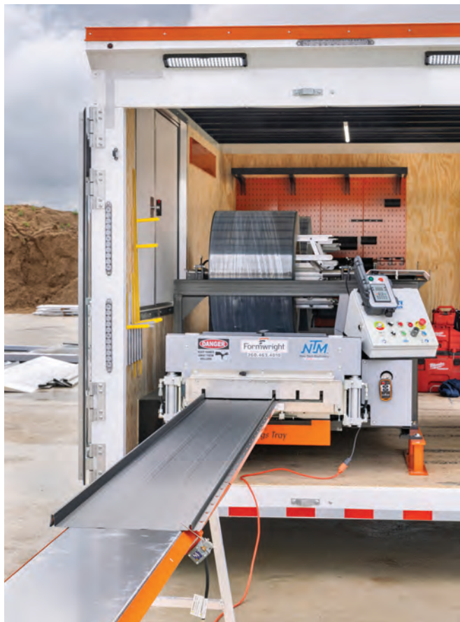
Exposure to the elements is not a concern when a portable roll former is housed in an enclosed trailer. PHOTO COURTESY OF FORMWRIGHT.
