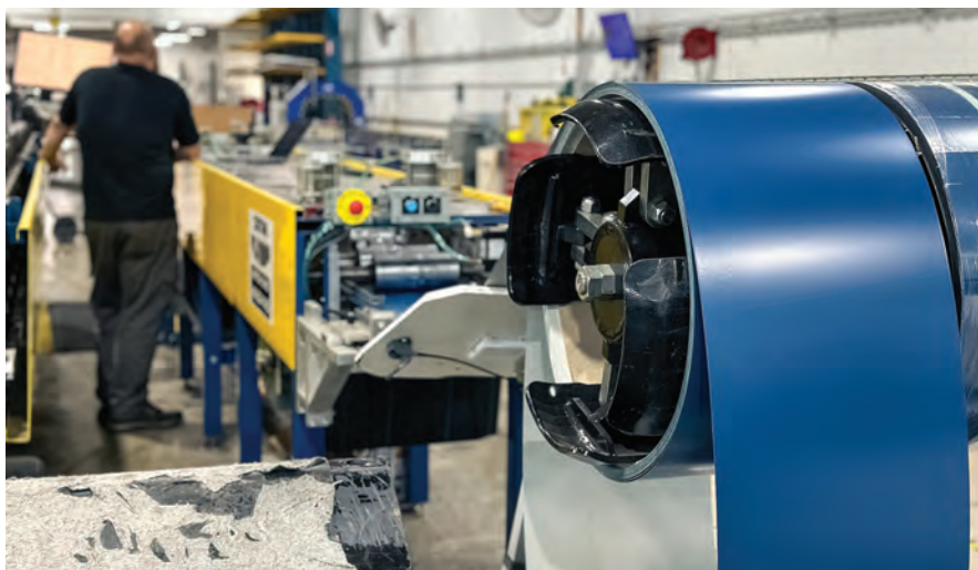
Metal Exteriors employee monitoring roll-forming line, where precision equipment transforms flat metal into finished roofing and siding panels.
