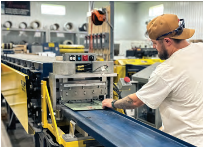
Panels are made on MRS roll formers.
