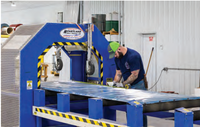
Panels are prepared for safe shipping using the wrapper from Heartland Sales & Machine.
