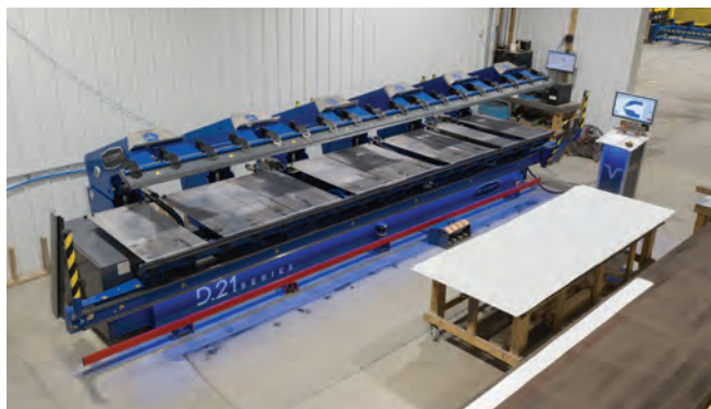
An aerial view of the Variobend 21' folder.
