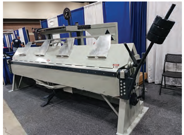
Stoll Metal Works offers low-tech affordable trim brakes and coil upenders, which are available in a variety of configurations to fit unique business requirements.
