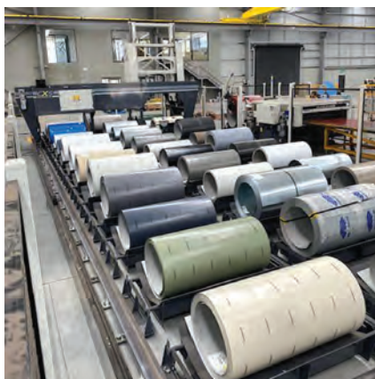
CX-5 Automatic Coil Changer: For higher volume applications. A CX5 coil farm can be coupled with most rollformers or SWI's Marxman Plus and Pro Slitter for fast, automatic coil changes. PHOTO COURTESY OF SWI MACHINERY
