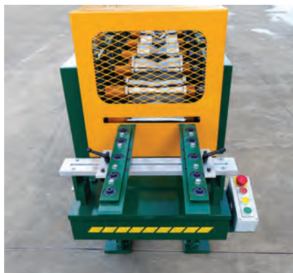
The F and J Trim Roll Former. PHOTOS COURTESY OF ACU-FORM
